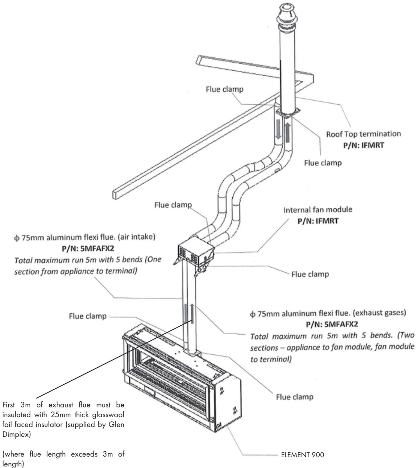
**Setup with internal fan module with rooftop termination – mid flue mounted**
