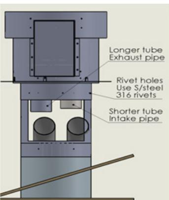
Fit the termination on to the access panel and match the rivet holes to rivet the termination to the access panel.
