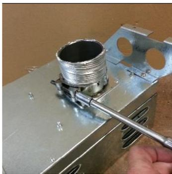
Turn fan assembly upside down and slide 65mm flue section fully onto spigot.
