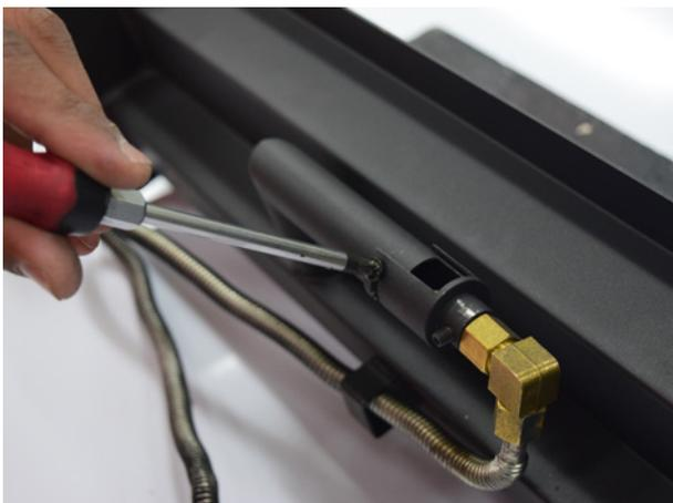
Refit injector assembly into aeration cap.
