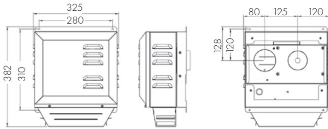
1. Wall mounted fan module – terminal must be installed with clearances as specified by AS5601.1 Clause 6.9.3.
