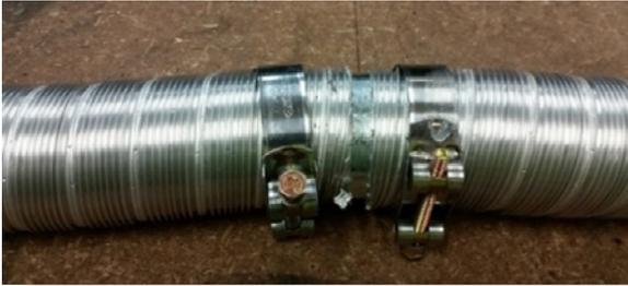
Slide each flue halfway onto connection joiner.
