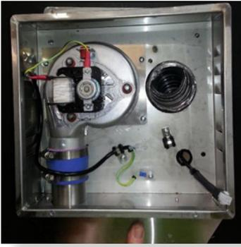
Assemble main body assembly onto wall mounting bracket, feed power cable through grommet hole prior to fitting. (refit 5 screws as shown and tighten) Main body assembly must sit flush up against the mounting bracket and seal.
