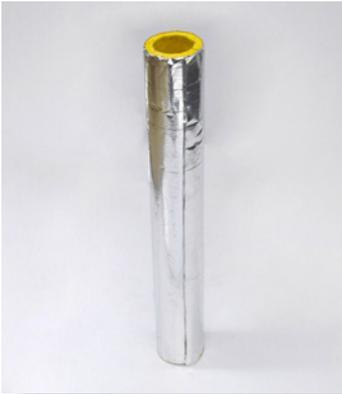
For all Element 900 installations using inline fan configurations (where flue length exceeds 3m), the first 3m (or up to 3m) of exhaust flue must be insulated with 25mm foil faces glasswool pipe insulation, as supplied by Glen Dimplex Australia.
