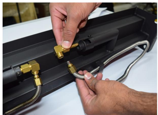
Loosen aeration cap screw approx. 1/2 turn. Rotate cap until the correct gap is achieved to suit the gas type. The listed opening is required on each side of the aeration cap. (A ruler or similar can be used to check the opening, a drill bit of the designated size can also be inserted to check the opening). Tighten screw to retain aeration cap setting.
