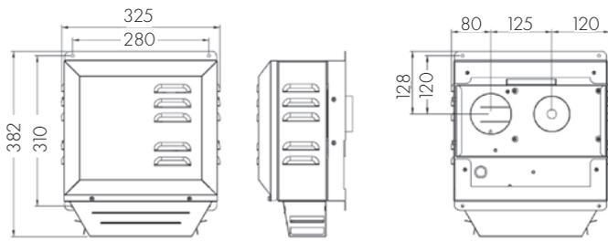
1. Wall mounted fan module – terminal must be installed with clearances as specified by AS5601.1 Clause 6.9.3.
