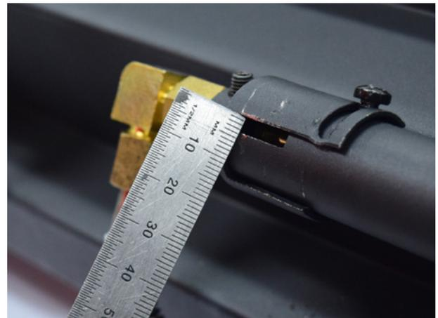
Rotate burner to check insulation is correctly located.
