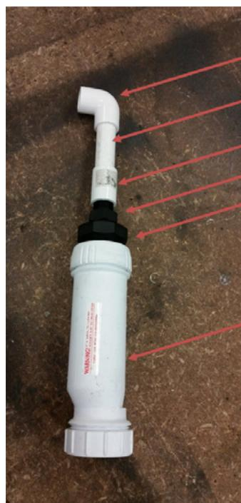
15mm PVC Elbow or 15mm STRAIGHT CONNECTOR
