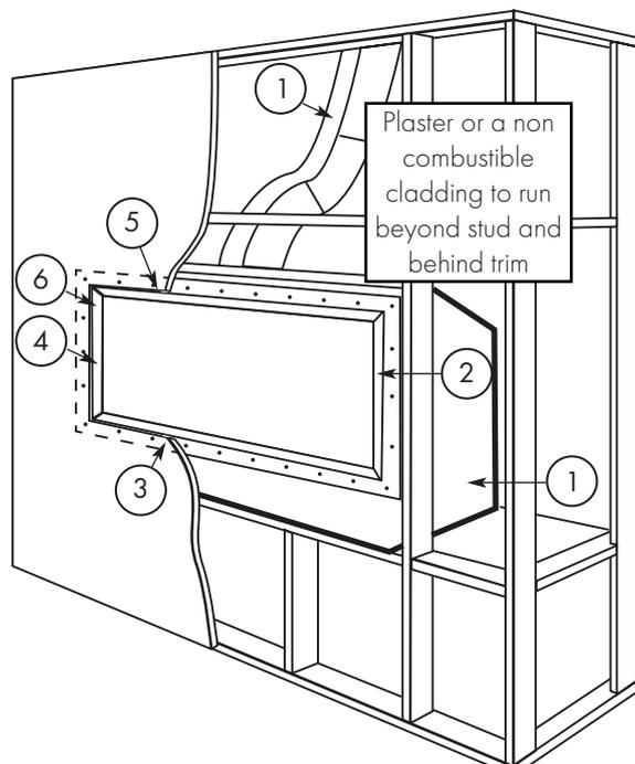
1. Install Element onto base and connect flue, gas and power.
