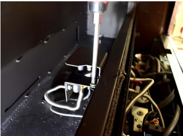
Remove pilot pipe fitting from pilot assembly.
