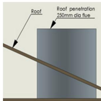
Insert the roof penetration and fix firmly to the roof structure using appropriate supports.
