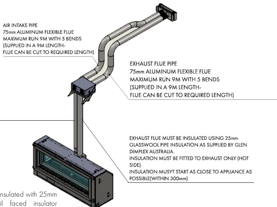
Exhaust flue must be insulated with 25mm
