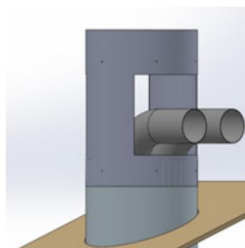
Run flue pipes through the access cut outs before fitting the termination on for ease of installation. (The picture is a reference only. Take care not to flex/bend the pipe too sharply and risk slitting the pipe)
