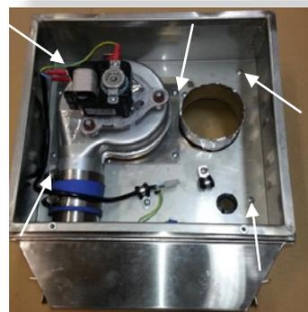
Remove the 5 screws as shown. (Do not remove fan plate screws)
