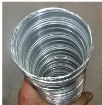
Check 75mm flue piece for correct shape and fitment onto appliance spigot.
