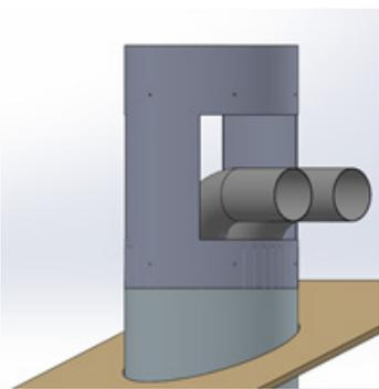
Run flue pipes through the access cut outs before fitting the termination on for ease of installation.
