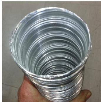
Run flue from appliance to bottom entry on fan module.
