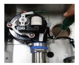
Push fan terminal into position. And affix to wall.
